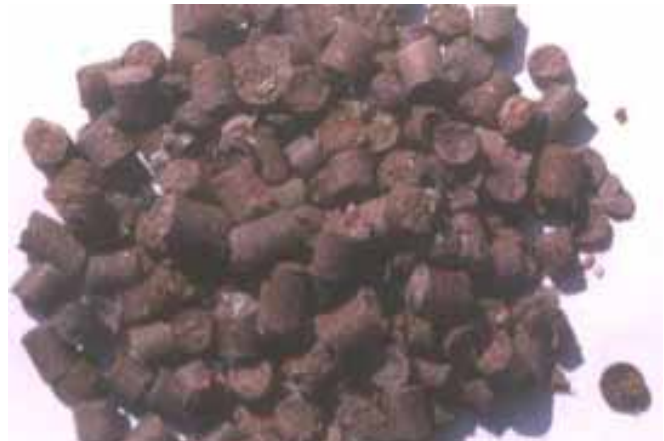
Densified RDF (pellet) Photo courtesy: Chamco.net
